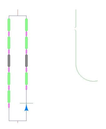
If you leave on the option to split the striprules to the knives, then the teeth close to the striprules are all removed, and the bridging centered between each set of striprules.
